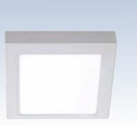
Pearl LED HPF flat panel comprises of aluminum die cast housing finished in white powder coated. The flat panel is pre-wired with high efficiency electronic driver. High translucent frosted PMMA diffuser is used to get glare free, smooth light distribution. This luminaire is recommended for surface mounting applications in general offices, institutions, retail shops, auditorium, & other commercial interiors replacing a traditional CFL downlighter.
