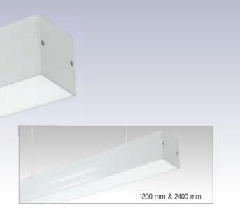
LED luminaire having 95 mm wide aluminum extruded profile finished in white powder coated. Snap fit high translucent frosted PMMA diffuser and high reflective aluminum reflector gives glare free light distribution with maximum efficiency. Another advantage of this system is the complete flexibility of continuous mounting which makes it adaptable to any architectural requirement and has a feature of overlapping lamp placement which results "shadow free" illumination.
